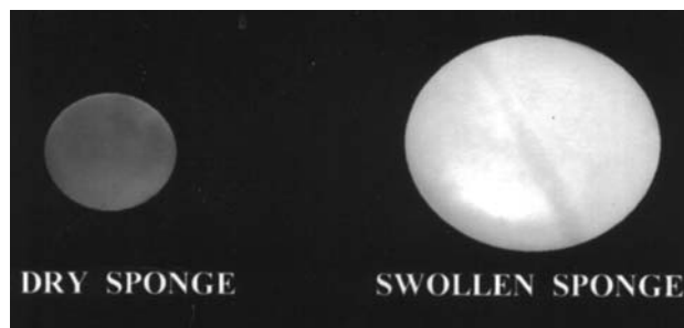
Fig. 1 A photograph showing the dry and swollen images of the semi-IPN
